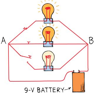
In contrast to a series circuit, the parallel circuit is completed whether all, two, or only one lamp is lit.
