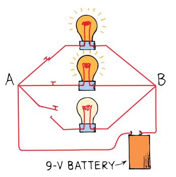
In this parallel circuit, a 9-volt battery provides 9 volts across each activated lamp. (Note the open switch in the lower branch.)
